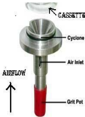
Figure 1; recommended silica sampling train
